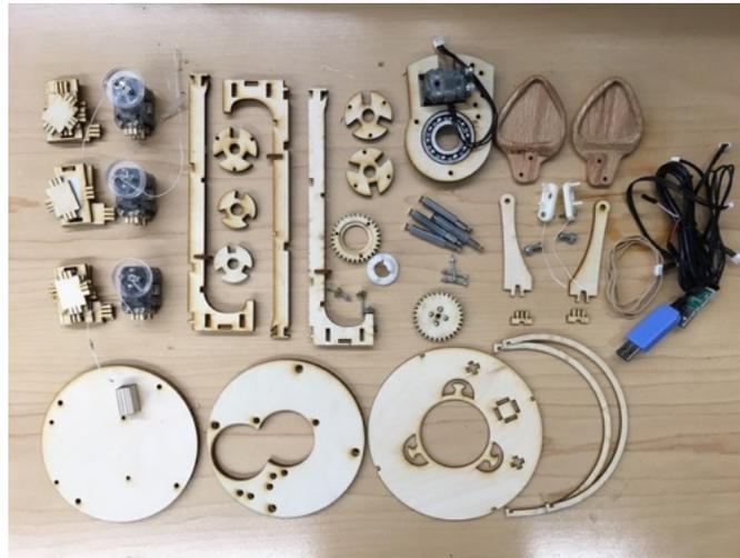
Figure 1.7: Layout of the components used to assemble the mechanism.
