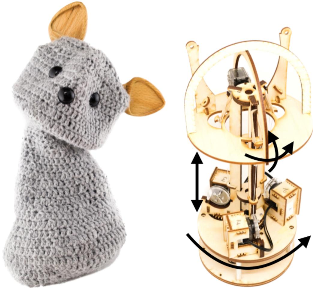
Figure 2.1: The Blossom robot. The exterior (left) is made of soft materials while the interior mechanism (right) consists of a central tower structure from which the head platform is suspended by elastic bands. The head platform has four degrees of freedom: roll, pitch, yaw, and vertical translation.
