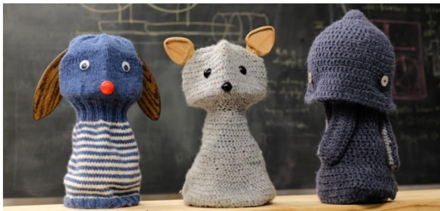
Figure 1.1: Three variations of Blossom with different embodiments and accessories. The robot on the left is knitted, and the two robots on the right are crocheted. The two robots on the left display swappable wooden ears and a number of attachable facial features, while the robot on the right features soft silicon arms as appendages.
