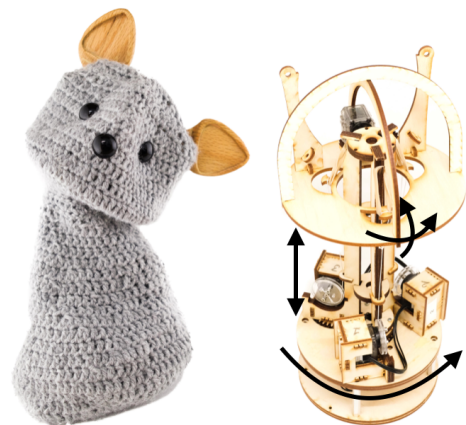
Figure 1: The Blossom robot. The exterior (left) is made of soft materials while the interior mechanism (right) consists of a central tower structure from which the head platform is suspended by elastic bands. The head platform has four degrees of freedom.
